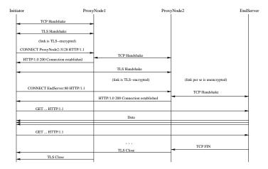
Fig. 2. Protocol run for a scenario where the initiating user builds a two-hop tunnel, fetches web site, and then closes the connection
