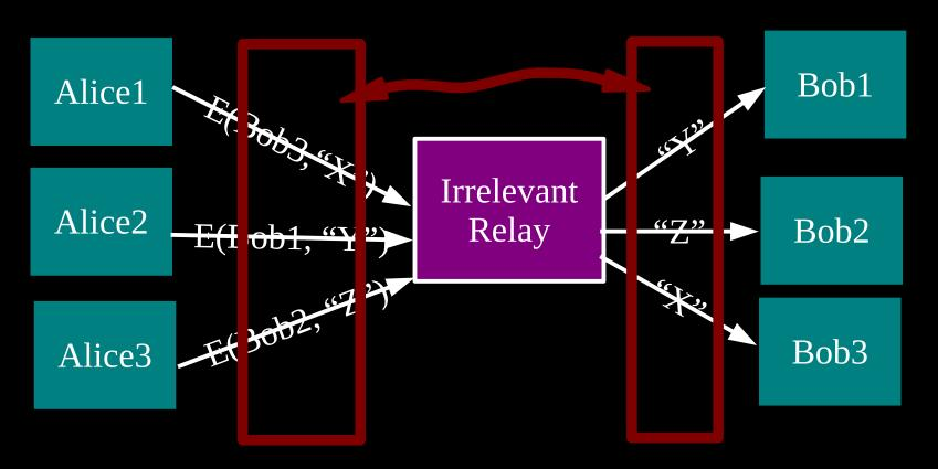
Timing analysis bridges all connections through relay ⇒ An attractive fat target
